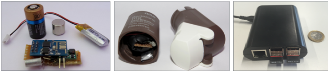
Fig. 3: Object Tags, (a) ESP SoC construction for a Mobile Object Tag, (b) An instrumented Inhaler with a Mobile Object Tag and (c) Raspberry Pi 2 Model B based Static Object Tag with two WiFi interfaces.
