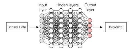
Fig. 2. Typical Deep Neural Network structure with feed-forward fully-connected layers.
