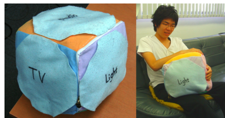
Figure 1: Visual appearance of C^3 . C^3 can be used both as a cushion and as a controller. The physical body is visually appealing and suitable for living spaces like everyday objects.
