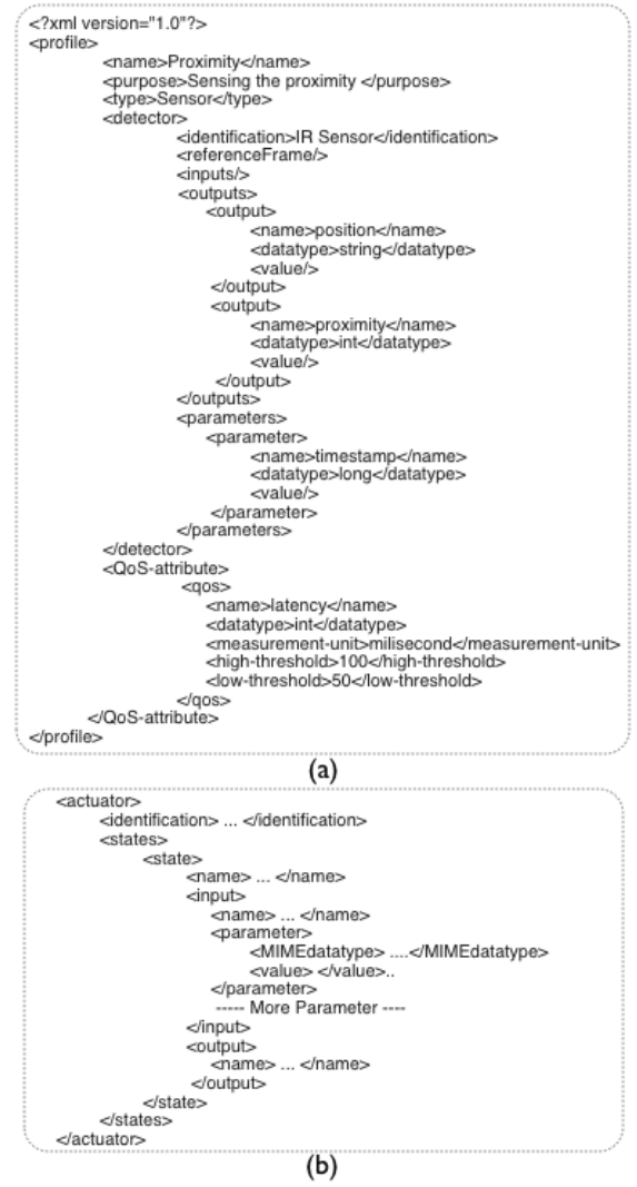
Figure 6: (a)Profile Description File for Proximity Profile . SensorML is used in the <detector> node. (b) Artefact Control Language is used for actuator profile, only the <detector> node is replaced with <actuator> node.
