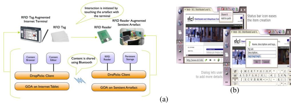
**Fig. 2.** (a) Architecture of DroPicks. GOA handles group management and RFID is utilized for initiating the communication (b) User Interfaces for Creating Content Items.
