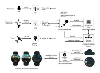
Figure 1: On-Wearable Interruptibility Management System
