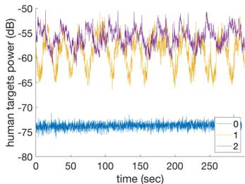
**Figure 6:** Aggregate human target power levels for moving people indoors across three occupancy cases.
